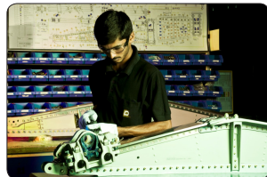
Assembly of Flap-Track-Beams for Airbus A320 Single Aisle Aircraft at Dynamic, Bangalore, India
